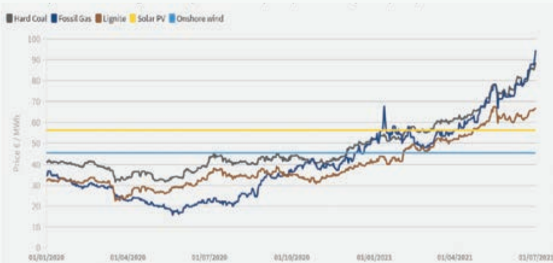
SIBIC calculated using Dutch TTF day ahead gas prices; EU ETS first December contract prices; APO Rotterdam front month prices; lignite fuel costs €1.5/MWh. Variable operating & maintenance costs €2/MWh. Plant efficiency factors: Hard coal = 38%; Lignite = 37%; Gas = 55%
